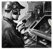
ALL LANDINGS were made with the aid of war-developed, radar ground-controlled approach units. These units plotted the planes over the field — 'talked' the pilot into position over the runway – then safely down to the ground. In two years, there wasn't a single accident. Lessons learned will mean safer, more comfortable civilian flying for you.
